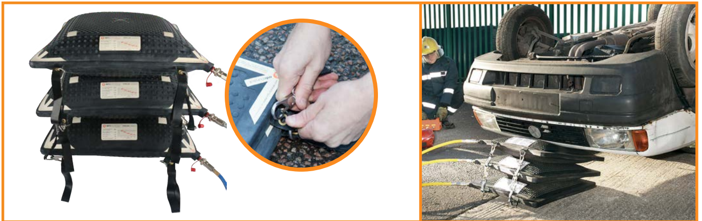
Fig 5.20: Combining Stak Jaks to increase lifting height
